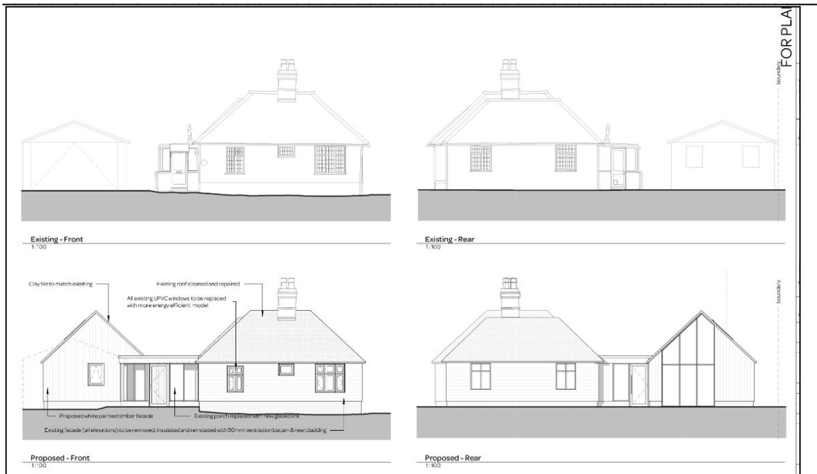
Figure 4: Existing and proposed front & rear elevations
